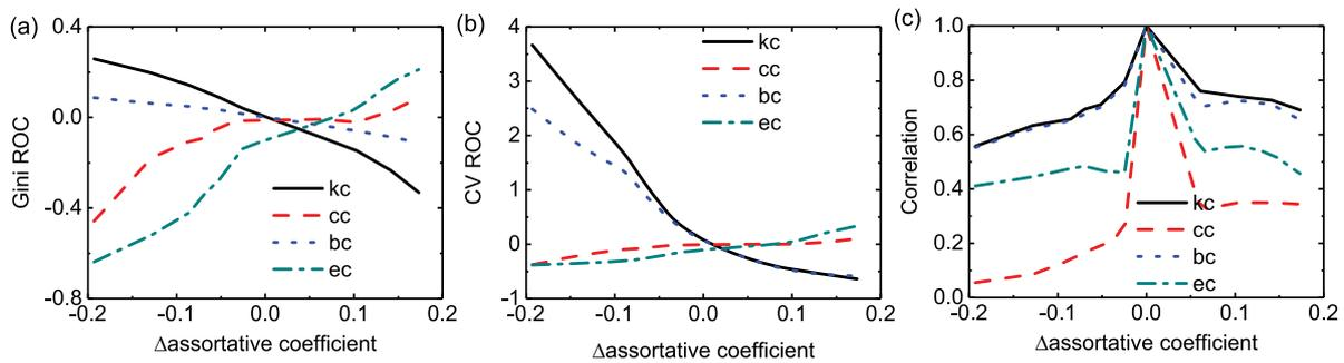
Fig. 2. Four centrality measures in the scale-free network model with tunable assortative coefficient. The cluster coefficient of these tunable assortative networks is that the mean value equals 0.447, and the standard deviation equals 0.112. (a) ROC of the gini index. (b) ROC of the coefficient of variation. (c) Correlation.
